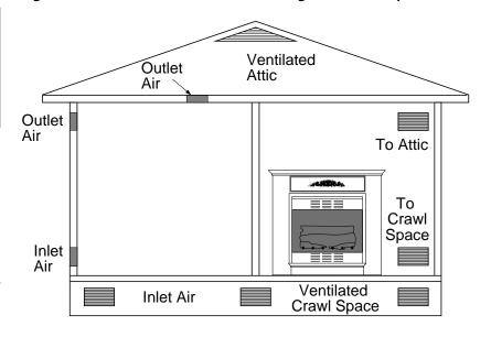
Figure 3 - Ventilation Air from Outdoors Shown with Optional Mantel
